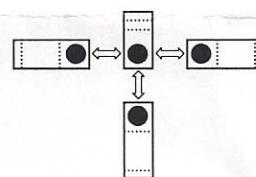
Switch is in the centre with magnets indicating each of the three possible operating positions.
